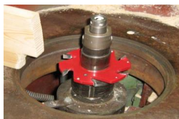
Figure 4. Spindle with fitted cutter
