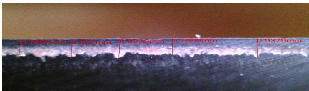
Figure 10. A picture of the flank wear width on the blunted blade after performing the experiment
