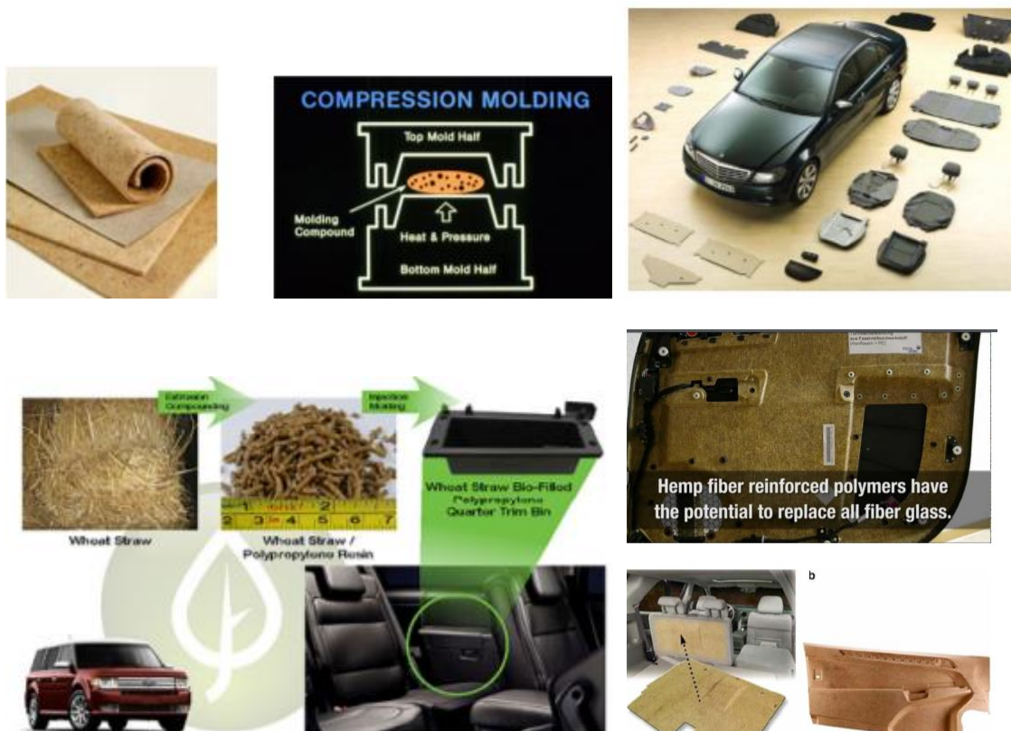
Figure 6. Hot press molding of automovie interior WPC parts
