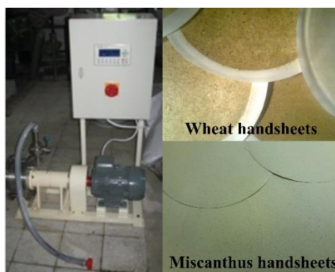
Figure 4. Hydrodynamic cavitation device and agro-waste paper handsheets
