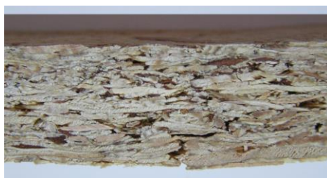
Figure 2. Standard deformation of the test specimens during testing the bending strength
