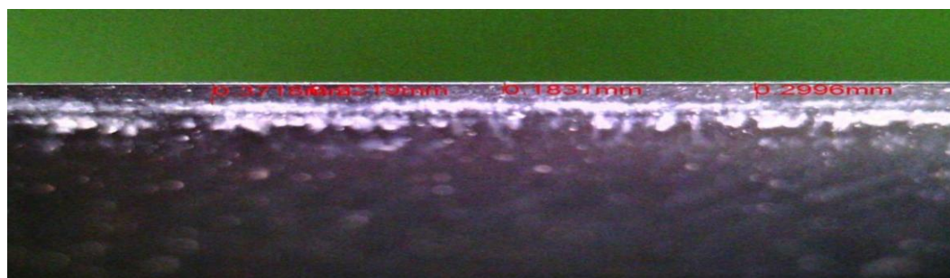
Figure 8. A picture of a flank wear width after the experiment on a newly sharpened blade
