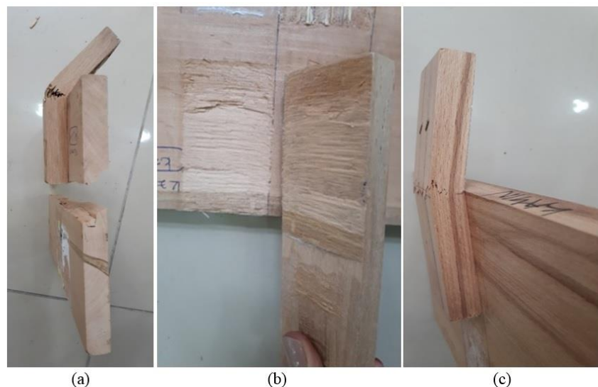
Figure 4. Failure modes of the joints with beech wood gusset-plate: a) failure with base member and gusset-plate rupture; b) separation from connection points; c) failure with gusset-plate rupture.
