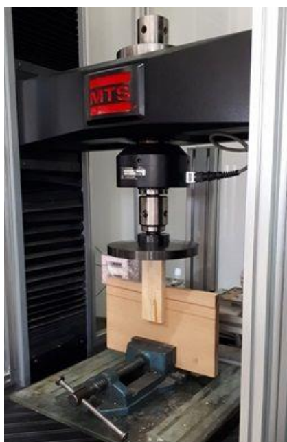
Figure 3. Test set-up for evaluating lateral shear load resistance of only glued gusset-plate joint.
