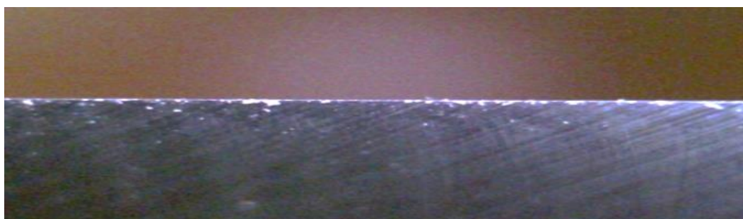
Figure 7. A picture of a flank wear width on a newly sharpened blade
