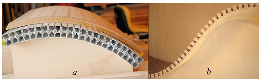
Figure 1. a - glue bent lamination; b - kerf bending
