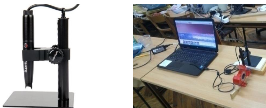
Figure 5. Digital microscope connected to a computer and the microscope
