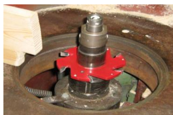
Figure 4. Spindle with fitted cutter
