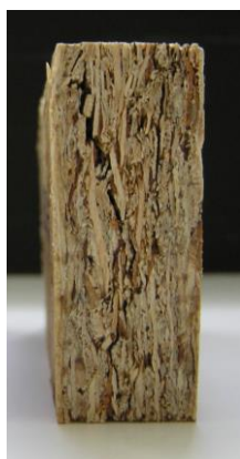
Figure 4. Standard deformation of the test specimens during testing the compressive strength
