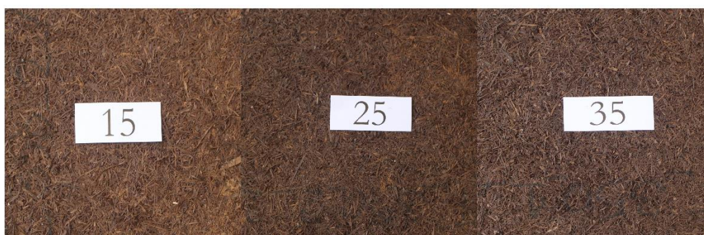
Figure 1 Panel appearance and formability after 15 h, 25 h and 35 h heat treatment
