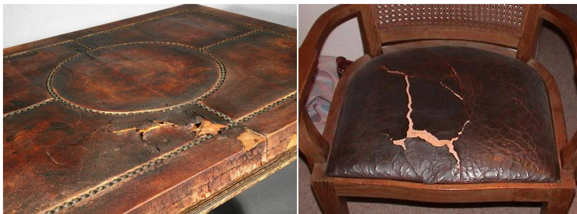
Figure 1. Furniture with dehydrated and damaged leather
